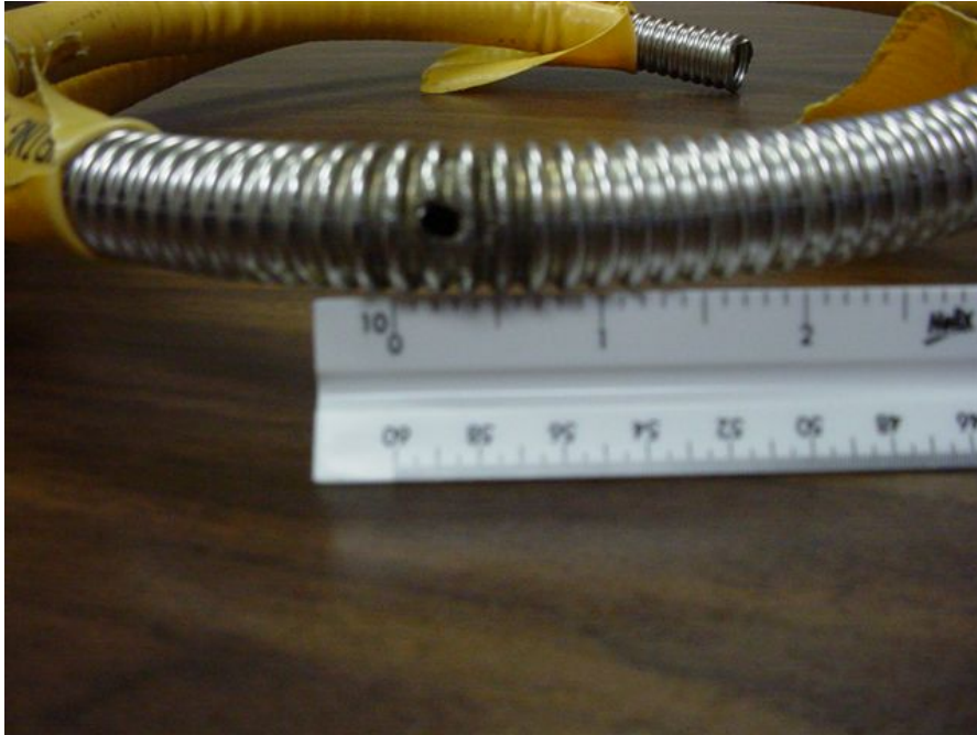
Figure 1 Typical Lightning Damage to CSST
